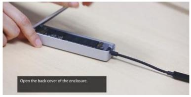
**Step 4**Use the T5 screwdriver to remove the screw holding the JetDrive SSD.
