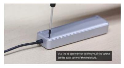
**Step 3**Open the back cover of the enclosure.
